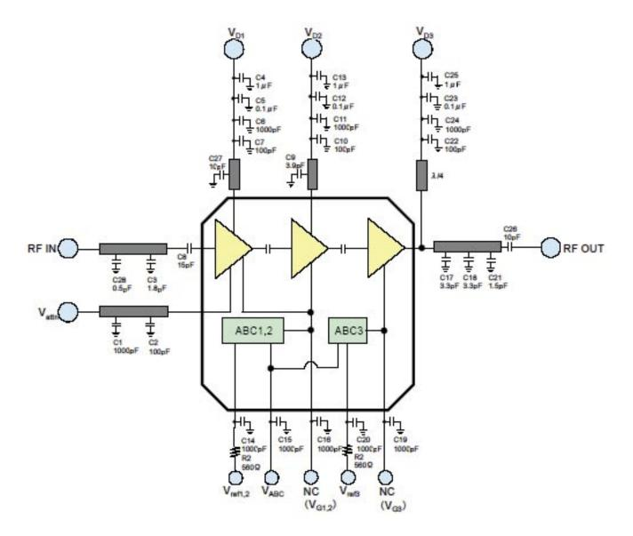
NC (VG1,2 VG3) These pins must be connected to ground via a 1000pF capacitor for stability.
